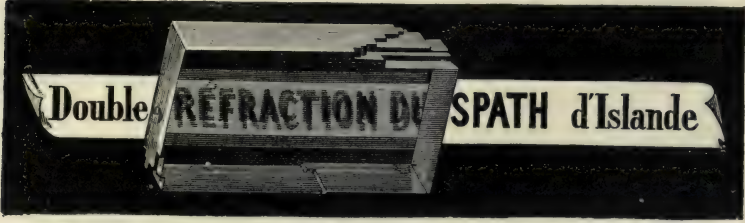
FIG. 108.—Double images seen through Iceland spar.
